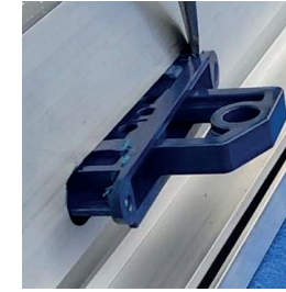
4. Pry the housing out using a screwdriver
