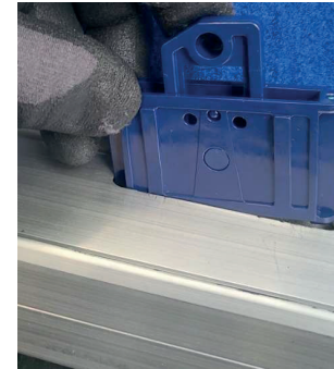
5. Insert the new Klick-Klack locking mechanism in the correct position in the slotted hole and alternately hammer left/right with a rubber mallet
