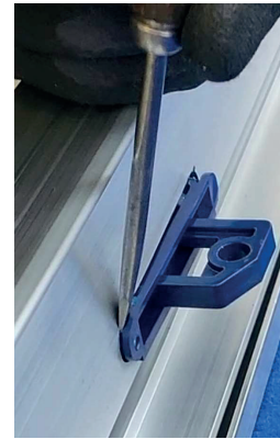
4. Pry the housing out using a screwdriver
