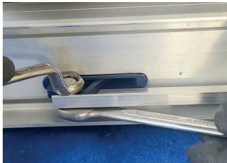
2. Loosen screws and nuts using an open-end spanner
