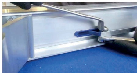
2. Loosen screws and nuts using an open-end spanner
