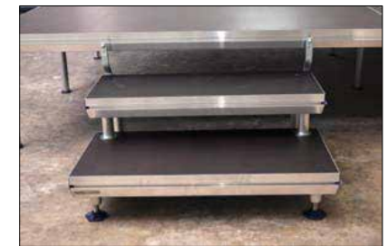
connection of stairway and stage (groove profile): 1 leg link 110 mm + 1 link N-F or 2 links N-F
