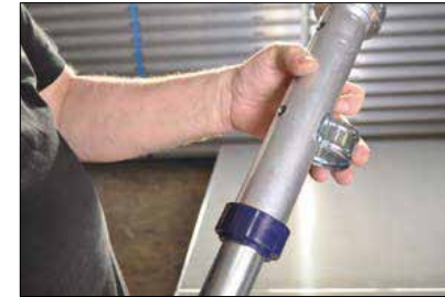
lock with safety bolt clip
