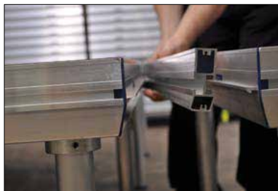
attachment of stairway at tongue profiles
