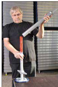
put interchangeable leg on spindle
