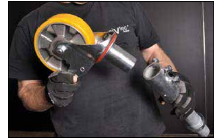
insert wheel into extension adapter and fasten safety screws
