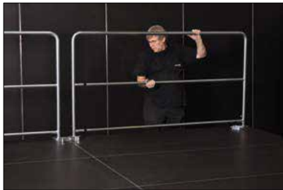
put on rails at the back fasten safety screws
