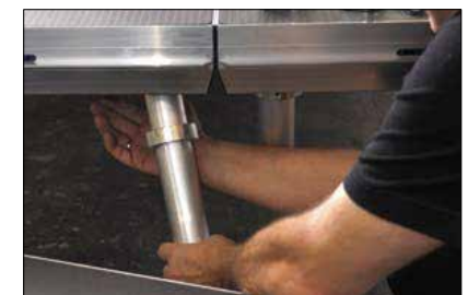
if necessary mount additional leg
